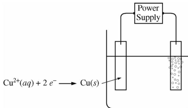
An external direct-current power supply is connected to two platinum electrodes immersed in a beaker containing 1.0 M  $\text{CuSO}_4(aq)$  at 25°C, as shown in the diagram above. As the cell operates, copper metal is deposited onto one electrode and  $\text{O}_2(g)$  is produced at the other electrode. The two reduction half-reactions for the overall reaction that occurs in the cell are shown in the table below.
